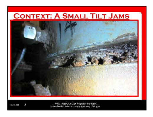
The context of bolted flange separation to install BOPs, well maintenance or brownfield tie ins:
